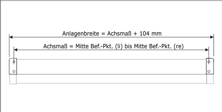
KONSOLE LINKS MONTIERT AUSSEN
